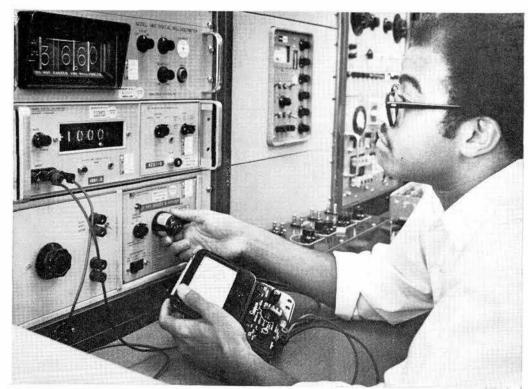
ELECTRONIC APPRENTICE Adrian Jones is calibrating a Simpson volt-ohm meter. The apprentices spend two different periods in the Instrument Repair and Calibration Section during their extensive training.
